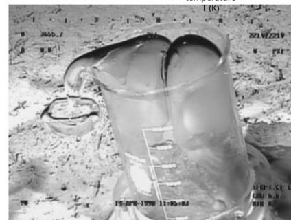
Fig. 5. Overflow of liquid CO 2 from the 4-liter beaker onto the sea floor at a 3650-m depth. A mass of transparent hydrate (CO 2 ·5.75H 2 O), formed at the upper interface, sank to the bottom of the beaker and pushed out the remaining liquid CO 2 . Ejected liquid CO 2 was highly mobile and did not appear to penetrate, or interact with, the sediments.
